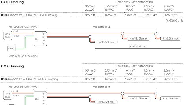
R014 + 200W PSUInstallation Guide – Wiring
